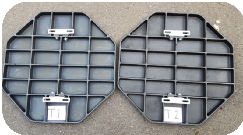
Figure 6: Photos of the backside of the rubber sign moulds T1 and T2.
