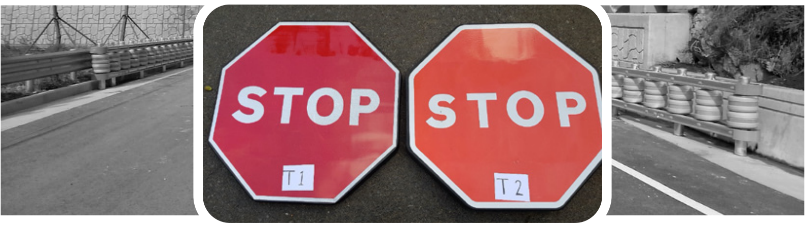
Figure 5: Degradation of rubber signs with different class retroreflective material.
