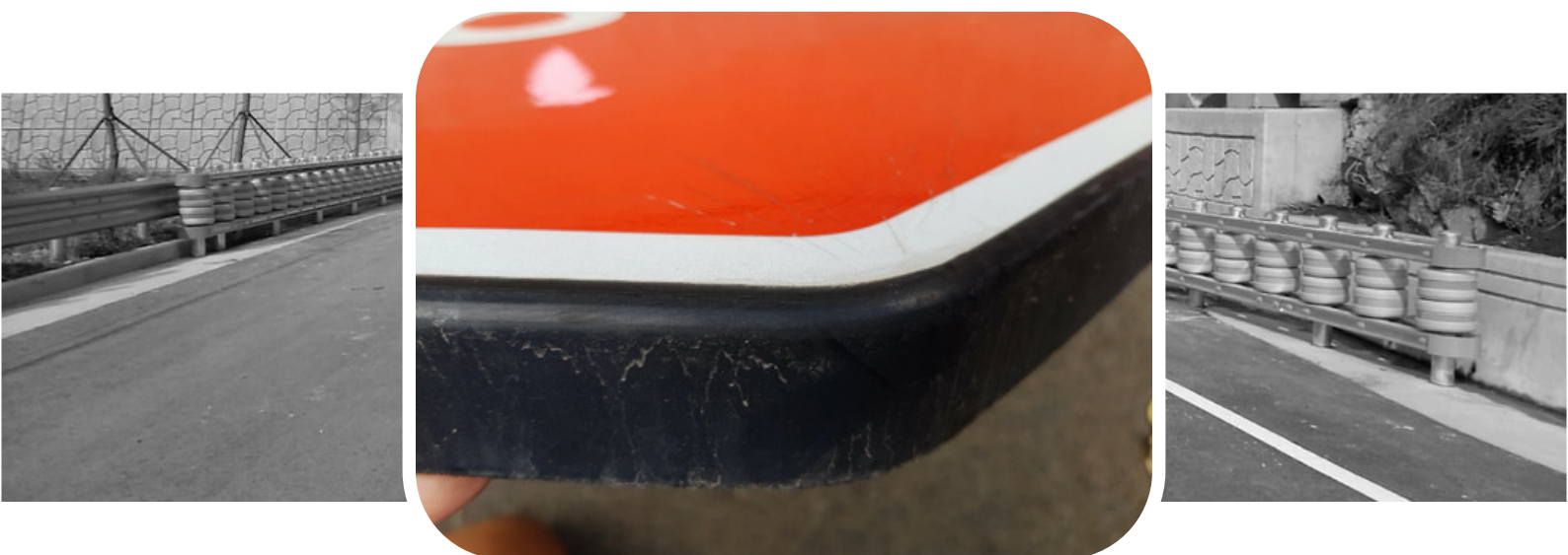
Figure 8: Photo of the delamination inspection between the retroreflective material and the rubber mould. No delamination was observed after 6 months.
