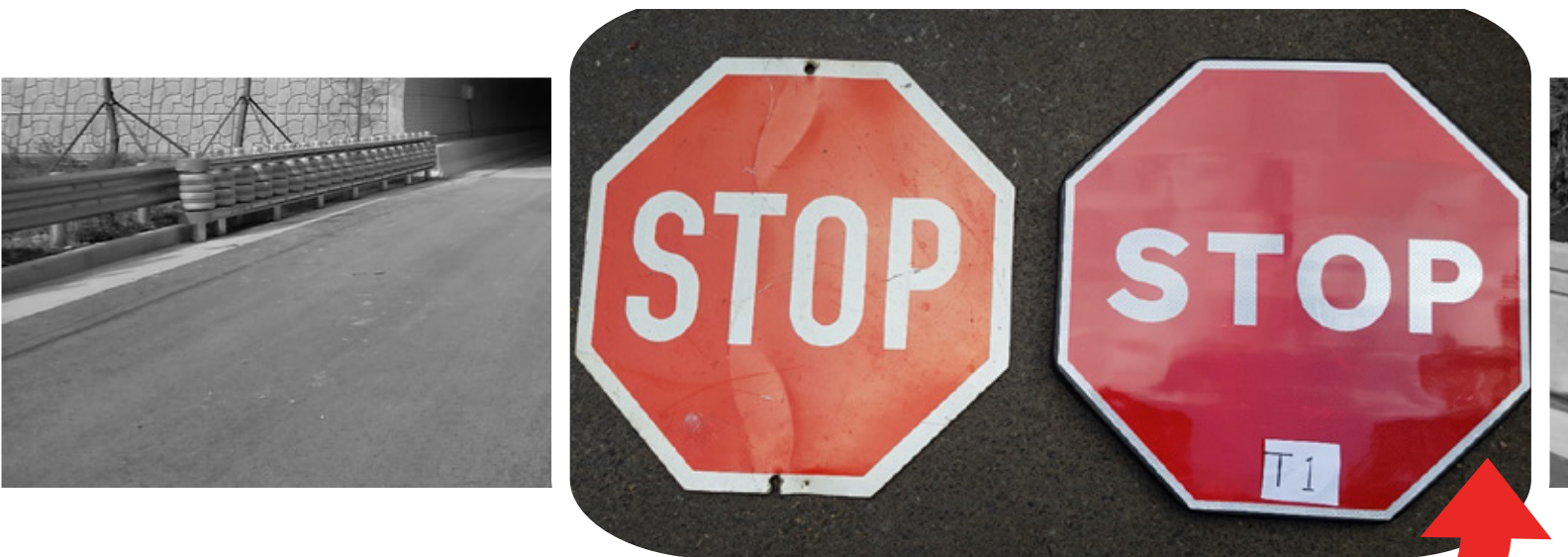
Figure 1: Compliant sign on the left, sample rubber sign on the right.
